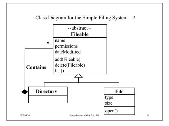
Structurally, this allows the same nested hierarchies of Fileable objects as the previous diagram. In this version, the "container-ish" methods (add(), delete(), and list()) have been placed on the most generic class, i.e., Fileable, rather than on the class Directory. This provides a uniform means of dealing with hierarchies of Fileable objects. A consequence is that File objects must ignore these methods or throw an exception.
