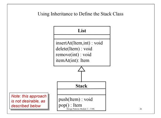
There are two flaws with using inheritance to implement the Stack class.
