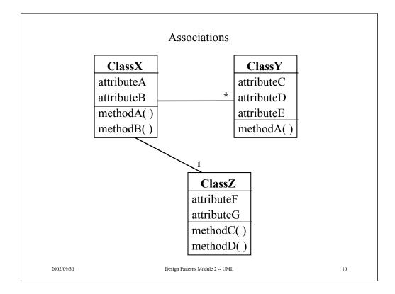
The asterisk (\*) shown at the right-hand end of the top line above means that the association involves zero or more instances of the attached class.
