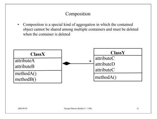
The notation in the diagram above indicates that an instance of ClassX has (or *is the parent of*) zero or more instances of ClassY, with the additional constraints that
