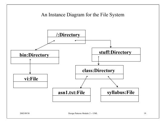
This instance diagram shows one (of an unlimited number) of the possible sets of Fileable objects that can be created that satisfy the class diagram on the previous page.
