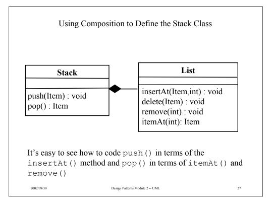
The composition approach is clearly superior to the use of inheritance in this case.
