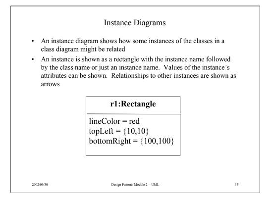
An instance diagram can be very useful to illustrate the associations that have been defined in one or more class diagrams. This usage supports the concept of walking through a scenario to validate the model.
