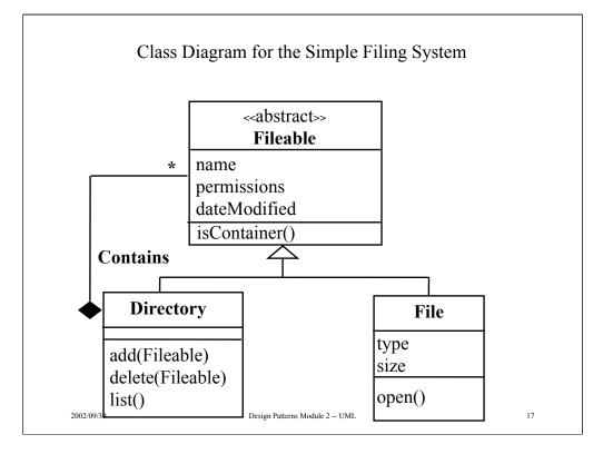
Note that with the interaction of the inheritance relationship and the aggregation relationship, the model defines arbitrarily deep instance hierarchies, as shown in the instance diagram on the next slide.
