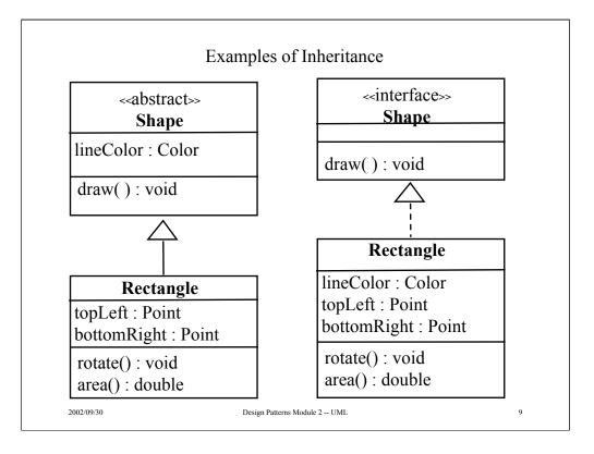
The left diagram shows class Rectangle extending (in Java-speak) class Shape. The Shape class shown has a very limited interface. The attribute lineColor is public and has two related public access methods: getLineColor() and setLineColor().
