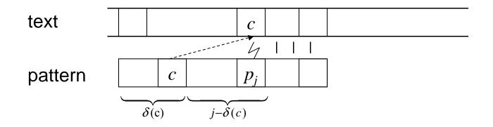
Shift the rightmost *c* in the pattern to *c* in the text.
