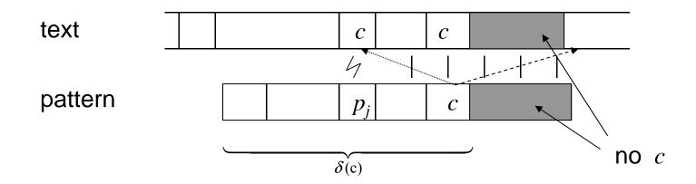
Shift the rightmost *c* in the pattern to a potential *c* in the text.
