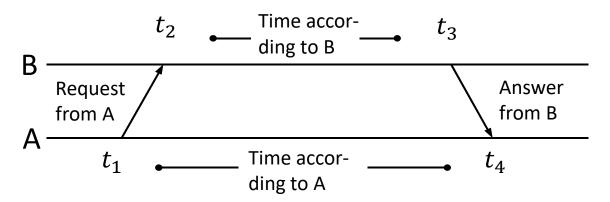
• Propagation delay  $\delta$  and clock skew  $\Theta$  can be calculated
