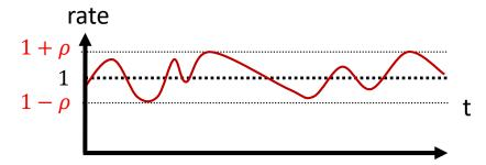
E.g., TinyNodes have a max. drift of 30-50 ppm (parts per million)
