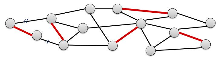
Maximal Matching: A matching s.t. no more edges can be added
